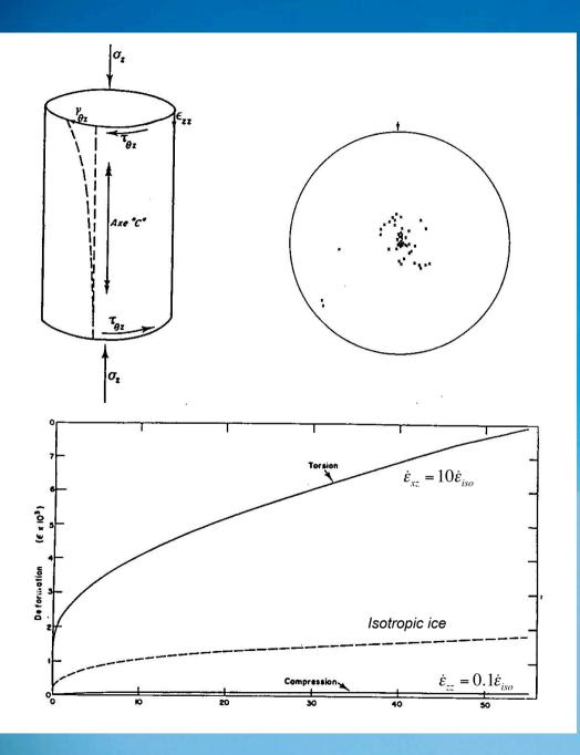
Viscosity of anisotropic ice: experimental measurements
