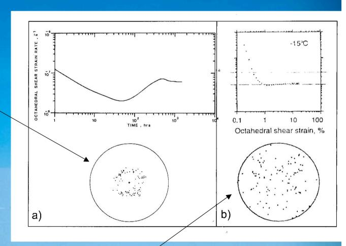
Strain less 20% is not enough high to form significant deformation textures
