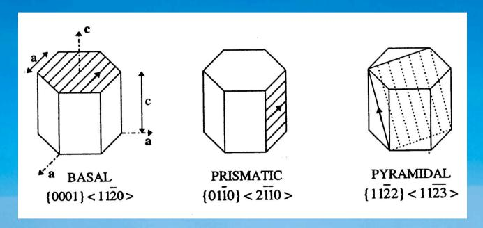
The shear strain rate on the slip system s, is:  $\gamma_s = \gamma_o \left| \frac{\tau^s}{\tau_o^s} \right|^{n_s - 1} \left( \frac{\tau^s}{\tau_o^s} \right)$
