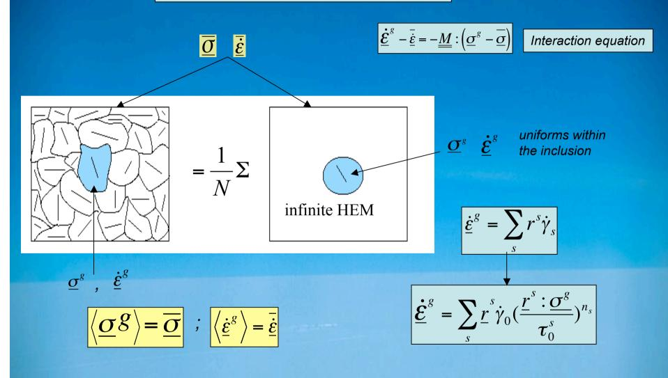
Local linearization of the stress against strain-rate response in the vicinity of overall stress and strain rate
