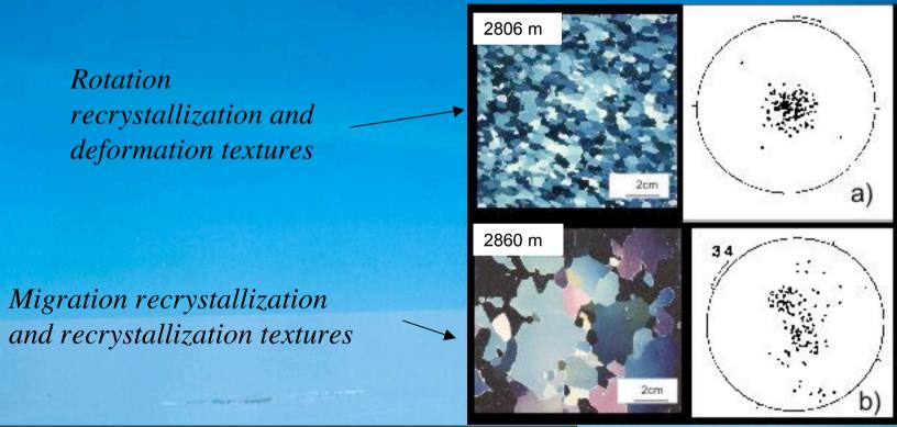
These two recrystallization regimes are observed at about the same depth along the 3,100 m GRIP ice core; variations of the impurity content would be at the origin of these two recrystallization processes
