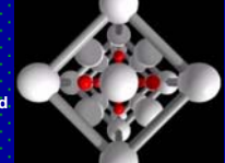
Zincblende ZnS. First structure solved by Braggs in 1913.
