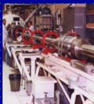
Shock-wave gun Caltech, LLNL: P < 500 GPa Snezhinsk: P < 10^4\text{--}10^5 GPa
