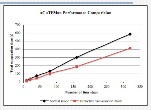
Total compute time reduced on average by 30 % Local disk space on Supercomputer also reduced
